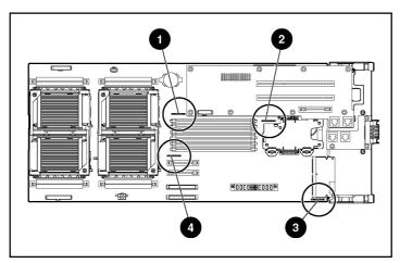
Figure E-2: System board LEDs
